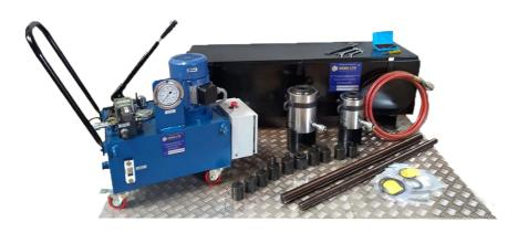
Single acting return hydraulic jacks are available in both alloy steel and aluminium. They have a 50 and 100mm stroke. Each pin, and bush can be replaced in one or multiple strokes. Jacks are centre hole type and are placed on C-sleeves (one over the other) through which the centre rod passes and nuts are tightened at the ends. Tie rods and nuts are machined from an alloy steel material, hardened, and tempered to increase strength and toughness.
