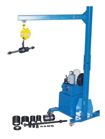
The trolley is an optional accessory that makes forenables the pin puller to have a precise and efficient operation
